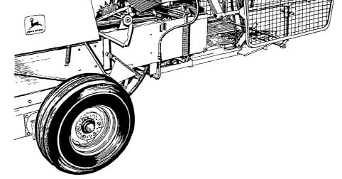
Two V-belts from the baler flywheel drive a pump in the Ejector's hydraulic system. Oil is diverted to a hydraulic cylinder which lifts the throwing pan to deliver bales to the wagon. There are very few moving parts.
