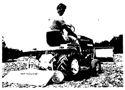
SPERRY NEW HOLLAND has introduced the 16 hp. Model S-16 lawn and garden tractor. Unit is available with a wide range of attachments including 54" front blade and 34" rotary tiller, shown.
