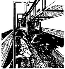
Model 166 Feeders are available for bunks from 50 to 200 feet long, are powered by a 1½ or 2 HP instant reverse motor.
