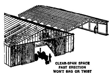
All the brute strength of curved steel is utilized throughout the exclusive framing system of Behlen's new "Tubeline" building. It's designed for strength, and for easy construction. Simple bolt-togsther connections speed erection. Clear-span design eliminates centerpole installation.
