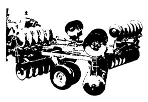
Fold-up models-15', 17', 19' and 21'-have positive, self locking wedge to hold gangs in working position. Fold up is fast and easy-no wrenches are required.
