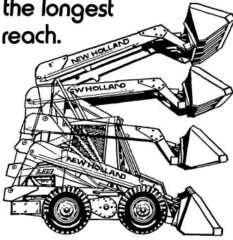
The New Holland Model L-35 utility loader reaches higher and farther forward than others in its class. It lifts more, too. Operating load (SAE) is 1,800 lbs. And you can change from buckets to forks to blade in seconds. Even converting to back hoe takes only a few minutes.
