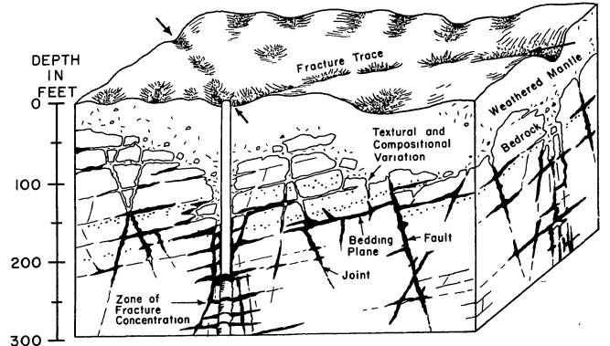
Nature's subterranean plumbing reveals itself by subtle lines on the earth's surface, normally visible only from the air. Two Penn State geologists spent 10 years perfecting the "fracture trace" method of prospecting for groundwater and
