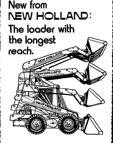
The New Holland Model L-35 utility loader reaches higher and farther forward than others in its class. It lifts more, too. Operating load (SAE) is 1,800 lbs. And you can change from buckets to forks to blade in seconds. Even converting to back hoe takes only a few minutes.
