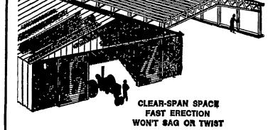
All the brute strength of ourved steel is utilized throughout the exclusive framing system of Behlen's new "Tubeline" building. It's designed for strength, and for easy construction. Simple bolt-together connections speed erection. Clear-span design eliminates centerpole installation.
