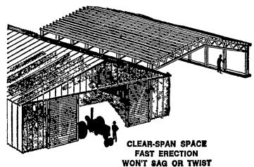
All the brute strength of curved size is utilized throughout the exclusive framing system of Behien's new "Tubeline" building. It's designed for strength, and for easy construction. Simple bolt-together connections speed erection. Clear-span design eliminates centerpole installation.
