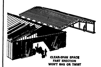
All the brute strength of curved steel is utilized throughout the exclusive framing system of Behlen's new "Tubeline" building. It's designed for strength, and for easy construction. Simple boit-together connections speed erection. Clear-span design eliminates centerpole installation.
