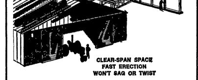
All the brute strength of curved steel is utilized throughout the exclusive framing system of Behlen's new "Tubeline" building. It's designed for strength, and for easy construction. Simple bolt-together connections speed erection. Clear-span design eliminates centerpole installation.
