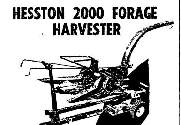
The 2000 features a 150 H.P. 1,000 RPM gear box and high capacity cutter. Can be used with a variety of Hesston Headers — 2 and 3 row corn headers, 2 row snapper header, and 6 ft. pickup header. Come in today and see this pull-type work horse.
