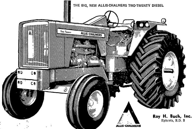
IT'S called the "LandHandler" because it's built for horizon to horizon farming. Walks right off with an 8-bottom plow, a 28-foot chisel, a pair of squadronhitched disc harrows and other big, wide implements.
