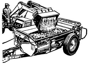
A hydraulic endgate of corrosionresistant steel matches the ruggedness of our New Holland spreaders. Rubber seals keep sloppy manure in. Linkage lifts endgate clear of heaped loads. Endgate is available for 130-, 163-, and 205-bushel single-beater spreaders. See them on our lot today!
