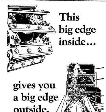
New Super 717 forage harvester has extra-strong, reinforced cutterhead that keeps chopping in toughest cutting conditions. It chops uniformly fine to 3/16". Choose from one-row, two-row standard or two-row narrow corn heads.
