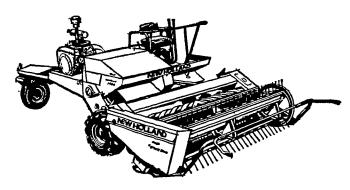
Self-propelled Model 1469 Haybine® mower-conditioner has 9-foot 3-inch cut and full-width, spiral rubber rolls. Keeps going when others plug! Two pull-type models also available: 7-foot 3-inch cut and 9-foot 3-inch cut.
