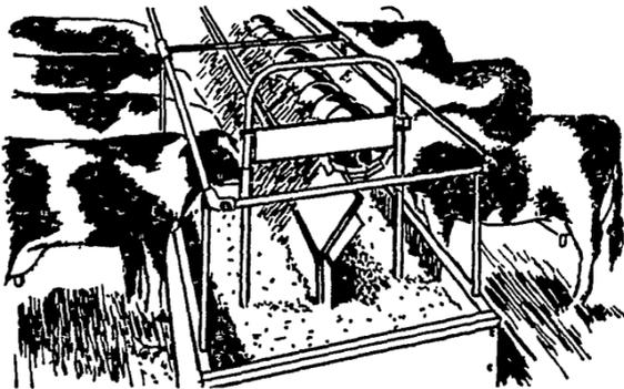
Hinged side of Jamesway Fill-N-Feed grain or silage feeder pulls away from J-trough and auger automatically to dump all feed fast...all at once without feed separation. All cattle get the same quality feed. Eliminates injuries from crowding, shoving.
