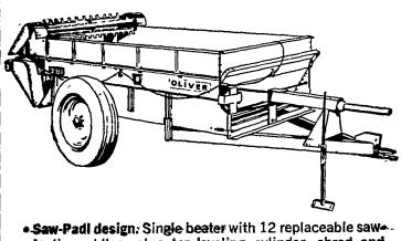
tooth paddles, plus top-leveling cylinder, shred and spread over a wide swath.
