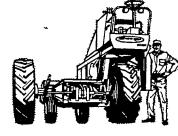
BIG NEW DIESEL POWER UNIT - 110 hp. Pick from 3 in all. Also 110 hp and 80 hp gasoline. All with good visibility, on-the-ground maintenance, adjustable seat and steering, power steering, individual hydraulic brakes.
