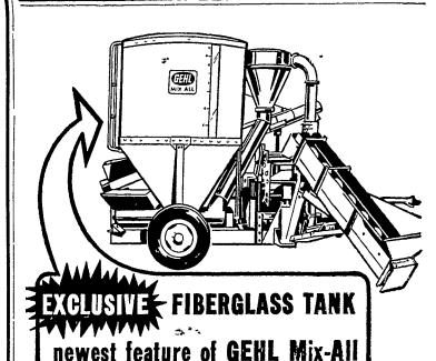
Another Gehl first! New, optional Mix-All tank of modern fiberglass reinforced plastic — the space-age building material. Advantages: tank is strong as steel, yet weighs 1/4 as much; rust-proof (not affected by salt or minerals); permanent molded-in white color won't scratch, peel or require re-painting, smooth interior sides reduce feed bridging, allow faster unloading; insulates better, reduces moisture condensation.
