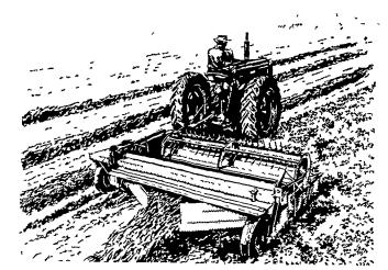
New Holland's new Haybine® mower-crusher sweeps through the tallest, thickest crops at up to 8 mph . . . producing an 8 ft. 9 in. swath (or a windrow) of fully-conditioned, fluffed-up hay. Whether you bale or chop your hay crops, you'll like the way the reel keeps the cutterbar clear, and practically eliminates plugging . . . even in tangled, downed crops! See this one-man haying machine now. Phone or stop in for a demon-
