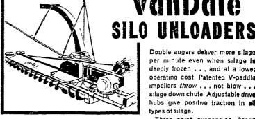
Double augers deliver more silage per minute even when silage is deeply frozen . . . and at a lower operating cost Patented V-paddle impellers throw . . . not blow . . . silage down chute. Adjustable drive hubs give positive traction in all types of silage.
