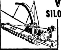
Double augers deliver more sliage per minute even when sliage is deeply frozen . . . and at a lower operating cost. Patented V-paddie Impellers throw . . . not blow . . . aliage down chute. Adjustable érive hubs give positive traction in all
