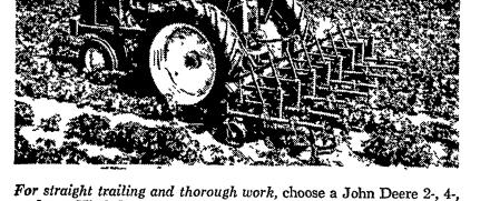
or 6-row Hitch-Mounted Cultivator. Each size mounts close to the rear of the tractor for easy handling. Large stabilizing coulters control drift on slopes. There's a full range of adjustments so you can position the tools for accurate, thorough coverage. RB and RG Series have square-tube frames; RR Series has double-bar angle-steel frame. Visit our store soon! We have a practical. confidential credit plan.
