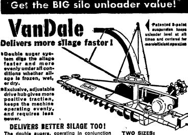
The double augers, operating in conjunction with the patented V-paddle impeliers, digs the silage, mixes it shoroughly, and then throws it down the chute. Your cows and cattle get good, palatable silage . . . not a powdered mash as seeften happens with unloaders using blowers.
