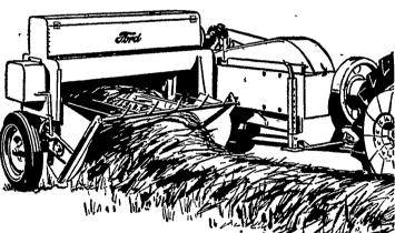
A PTO-driven, twine-tie baler that's both economical and efficient. Bales up to 5 bales per minute, or 8 tons per hour.
