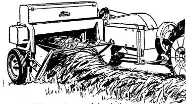
A PTO-driven, twine-tie baler that's both economical and efficient Bales up to 5 bales per minute, or 8 tons per hour.
