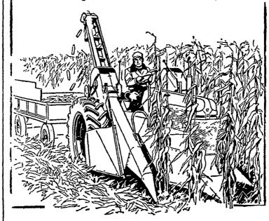
Here's your best choice of two-row mounted corn pickers. Long, eager snapping rolls with spacing you can adjust from the tractor seat. New roller-type gathering chains cut upkeep costs . . . are twice as strong, last three times as long as pressed steel or pintle types.
