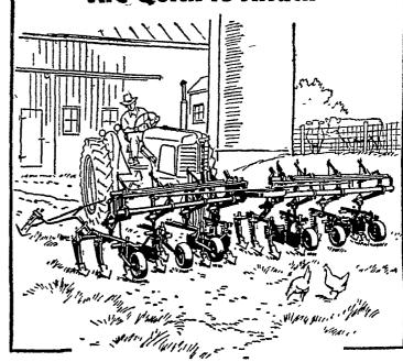
New "drive-in" mounted 2-row and 4-row cultivators for Oliver row crop tractors can be attached in a few minutes. Besides, they're interchangeable among the three tractor sizes, adjustable in row width from
