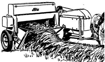
A PTO-driven, twine-tie baler that's both economical and efficient. Bales up to 5 bales per minute, or 8 tons per hour.
