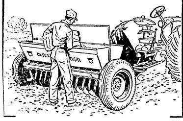
This new No. 64 Drill doubles capacity—holds a bushel of grain and 80 pounds of fercilizer per foot. The exstemely low hopper-cally 3/2 fect off the ground-is casier to fill. And, you have this same low height the har you choose 20-inch or 15-inch wheels, both islang low-cost, used tires.
