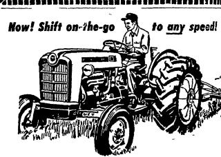
Hydraulic power does the actual shifting, but it's controlled by this handy lever under the steering wheel. A light touch is all you need to shift to any gear - 10 speeds forward, 2 reverse—at any time.
