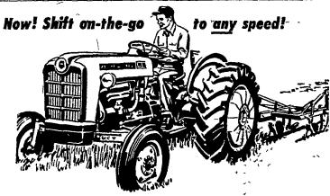
Hydraulic power does the actual shifting, but it's controlled by this handy lever under the steering wheel. A light touch is all you need to shift to any year - 10 speeds forward, 2 reverse—at any time.
