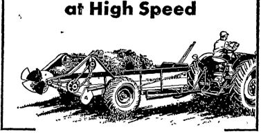
Heap it up! This Oliver No. 17 is rugged... shreds the big forkfuls from tractor loaders easily. A large main cylinder tears apart the matted chunks...the Hammermill Widespread distributes evenly over a full 7-foot
