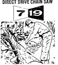
Homelite's new 7-19 direct drive chain saw is helping farmers turn their wood lots into money the fast leasy way. Cuts through 8 hardwood in 4 seconds 18" softs and in 12 seconds. Fells trees up to 5 feet in diameter Weighs only 19 pounds (less bar and chain) Straight blades plunge cut box trush cutter at tachments. Try it today!
