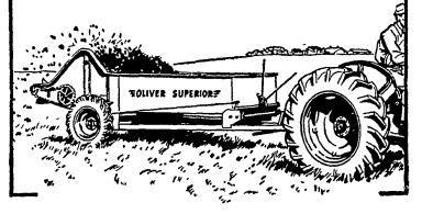
This 50-bushel No. 11 Spreader is handy...rugged... compact. It can be pulled and maneuvered by a small tractor-easily. And, a self-locking hitch stand eliminates heavy lifting. No jackscrews to turn.
