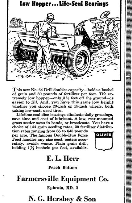
This new No. 64 Drill doubles capacity—holds a bushel of grain and 80 pounds of fertilizer per foot. The extremely low hopper-only 31/2 feet off the ground-is easier to fill. And, you have this same low height whether you choose 20-inch or 15-inch wheels, both taking low-cost, used tires.
