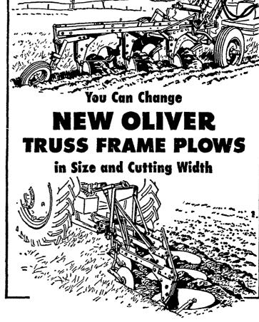
Both these new Oliver truss frame plows—the 2-3 bottom No. 4240 and the 2-3 bottom No. 3240 for 3-point hitches—are convertible. Add a bottom, take one off—or set them to cut 12, 14 or 16 inches—to suit field conditions, to fit your power. You can do it yourself easily-in a few minutes.
