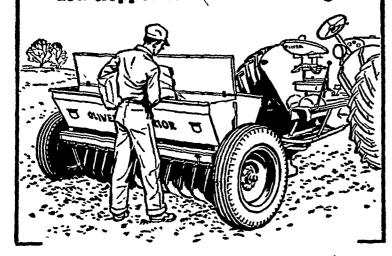
This new No. 64 Drill doubles capacity—holds a bushel of grain and 80 pounds of fertilizer per foot. The extremely low hopper-only 31/2 feet off the ground-is easier to fill. And, you have this same low height whether you choose 20-inch or 15-inch wheels, both taking low-cost, used tires.
