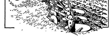
Both these new Oliver truss frame plows-the 2-3 bottom No. 4240 and the 2-3 bottom No. 3240 for 3-point hitches-are convertible. Add a bottom, take one off-or set them to cut 12, 14 or 16 inches-to suit field conditions, to fit your power. You can do it yourself easily-in a few minutes.
