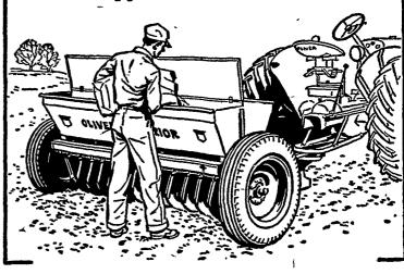
This new No. 64 Drill doubles capacity—holds a bushel of grain and 80 pounds of fertilizer per foot. The extremely low hopper-only 3½ feet off the ground-is easier to fill. And, you have this same low height whether you choose 20-inch or 15-inch wheels, both taking low-cost, used tires.
