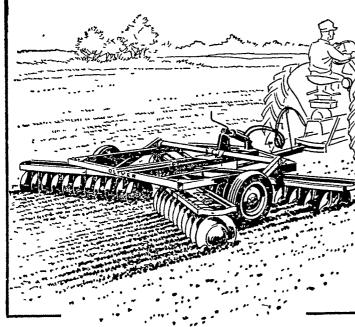
Built with adequate rigidity to penetrate the toughest soils, yet with sufficient flexibility to do a fine job in stony fields without damage to blades and frame Gangs are spring cushioned, permitting the new Oliver No 240 to ride over obstructions without being completely lifted out of the ground
