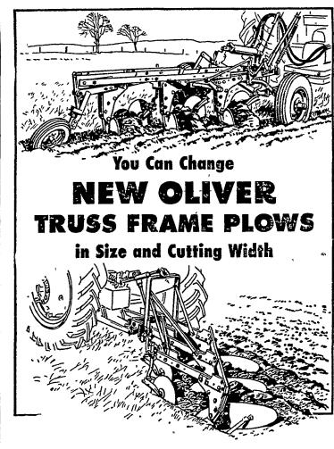
Both these new Oliver truss frame plows—the 2-3 bottom No. 4240 and the 2-3 bottom No. 3240 for 3-point hitches-are convertible. Add a bottom, take one off-or set them to cut 12, 14 or 16 inches-to suit field conditions, to fit your power. You can do it yourself easily-in a few minutes.
